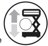
When lowering the platform, the platform should stop when it is approximately 2.1 m from the ground. Be sure the area below the platform is clear of personnel and obstructions before continuing. To continue lowering, release the control handle, wait 5 seconds, then move the control handle again.
