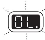
Flashing OL in the LED diagnostic readout indicates the platform is overloaded and no functions will operate. An alarm will sound.
