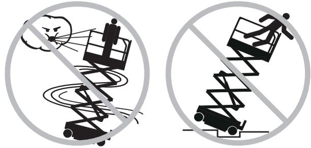
Use extreme care and slow speeds while driving the machine in a stowed position across uneven terrain, debris, unstable or slippery surfaces and near holes and drop-offs.
