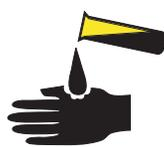
Avoid spilling or contacting battery acid. Neutralize battery acid spills with baking soda and water.
